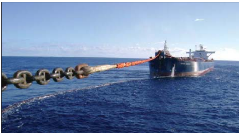
Tandem loading at Espadarte Sul field off Brazil with Aker Solutions' offshore loading system. Photo courtesy of Aker Solutions.
